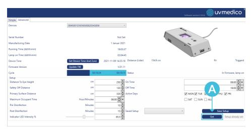
Once this information is saved and programmed into the unit, it is ready to test/start up. The unit will calculate the radiation automatically to stay within the limits of the ACGIH like the example below:
