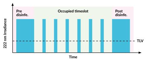
If during the duty cycle a person comes closer to the unit than the programmed distance from the eye, UV222 will automatically stop, and it will resume the activity 10 sec. after this security distance is cleared.
