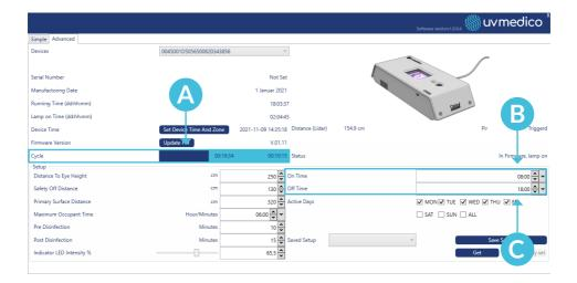
5) Add the pre and post cleaning cycle. D The unit will/can light up before and after the duty cycle so you can ensure it when people enter or leave.
